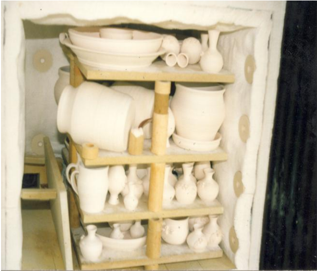
Kiln packed - Fired 1280 ° C
